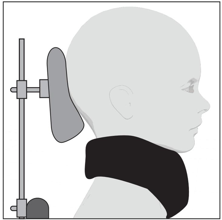
the top of a stiff neck collar and stretching the neck during a frontal crash. Since stiffer collars produced higher neck tensions, it is recommended to use the softest and lightest collar that can perform the needed medical function.
